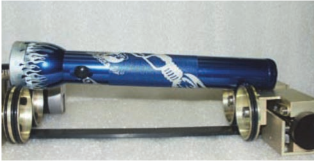
Incorrect Setup: The flashlight is not horizontal. Raise the right side of the flashlight by turning the jack screw.
